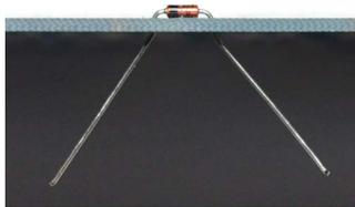
Flip the board over, solder the diode leads, then trim them just above the solder joint.
