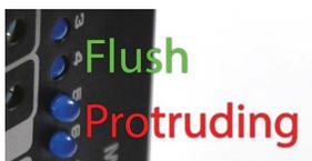
If you have LED spacers, just slip them onto the LED leads before stuffing them into the PCB and they will make sure the LEDs come out the right height.
