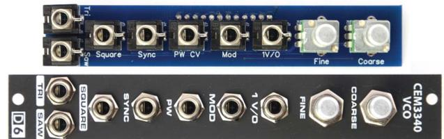
Solder the pots into place. Carefully snug all the nuts down using a socket.
