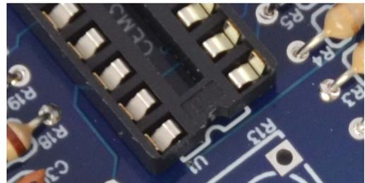
Flip the board over and solder one pin on each corner of the socket. This makes it easy to reposition the socket in case it isn't seated all the way down against the board; just reheat the corner pin and adjust the socket position as necessary.
