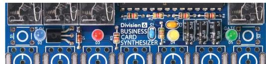
Insert the LED in the board, making sure that the polarity is correct (!) and that the spacer is flat against the board and the bottom of the LED. Solder, then trim the leads.
