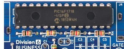
Flip the board over and solder one pin on each corner of the IC. This makes it easy to reposition the part in case it isn't seated all the way down against the board; just reheat the corner pins and adjust the position as necessary.
