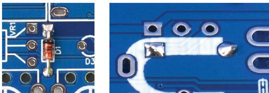
Note: For this build, we're going to be clipping the component leads a bit shorter than you may do normally to ensure that the board will fit inside the BC Synth enclosure if desired. Clip the leads as close to the solder joints as you can without cutting into the joints themselves.
